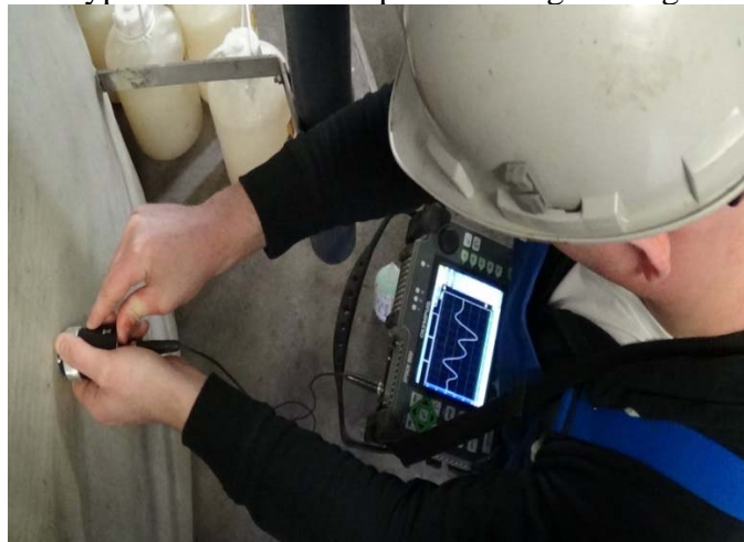
Figure 7. Typical view of a trained inspector taking ultrasonic readings on FRP tank.
