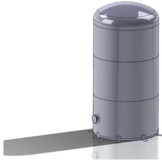
Figure 5. Configuration of Ferrous Chloride Tank. Ladder, overflow and some nozzles are not shown.
