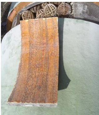
Photo 2: Cut Section with Corrosion Barrier Damage
